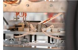
POST WELDING MACHINE With hot pin or Rotary burner tecnology Up and Down movement by servomotor Automatic adjustment of Fw/Bw movement of welding group Automatic adjustment of left/rigth position of welding group Automatic adjustment of giude widht Productivity: Up to 6 battery per minute Fast and easy change over High Performace / Durable and robust / User friendly / Easy maintenace machine **Optional**: Lead wire unwinder for truck battery
